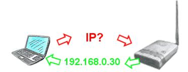
You use your PC in your company network with DHCP, so you dont have to care the everlasting setting of the ip-address. No problem, ALF also can be configured as a DHCP-server and assigns you accessing to the device via LAN or WLAN an ip-address from a predefined address range.
