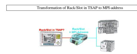
Your panel or visualisation system addresses the used PLC with Rack/Slot in TSAP? No problem, activate this mode in the S7-LAN and you will get actual data from the PLC.
