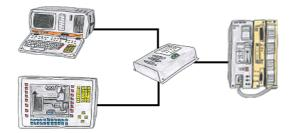
Your PD-interface of the S5-PLC is already occupied with a panel and you should accomplish program modifications without removing the panel? No problem, connect the Multiplexer one-time to the PLC and then connect the panel and also your PC to the Multiplexer. Now you can work parallel with the PLC without the need of affecting the operation of the panel.
