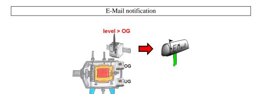
Do you monitor processes and upon reaching a predetermined upper/lower limit, you need a message? Then activate in the device the limit-value-monitoring and you get this message. Furthermore, the device also sends its state and you are always up to date.
