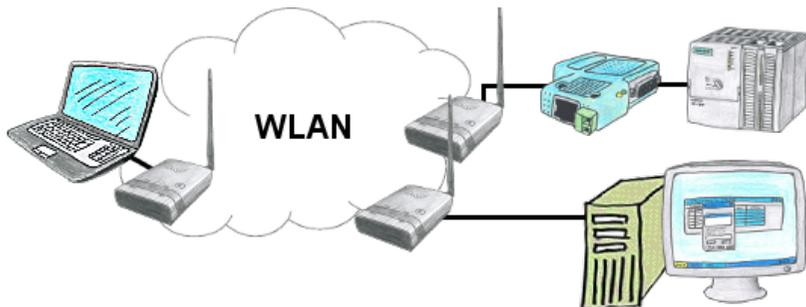
You have two or more clients which should communicate together without LAN-cable-connection? No problem, you connect a "Access-Point" configured ALF to this device and to the other device a "Client" configured ALF. Then connect the "Client" with the "Access-Point" and the device are able to communicate together.
