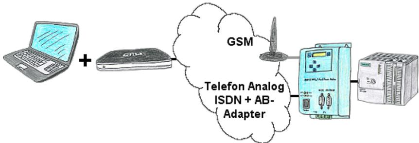
The access to the connected PLC with the Siemens TS-software or PG-2000 including TS-option results of coupling via Analogue-, ISDN- (only with AB-adapter) as well as GSM-line.
