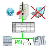
S7-PLC triggered DB-backup/-restore without additional PC via PN-port to USB-stick
