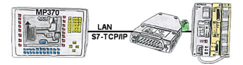
Your panel only has a LAN-socket as PLC-interface and supports only S7-RFC1006, no problem. Connect this socket with the S5-LAN++ and plug it directly on the PD-interface of the PLC. The S5-LAN++ performs adverse your panel as a S7-PLC although you receive the data from the S5-PLC. Then access to the variables and data of the S5-PLC is already available.
