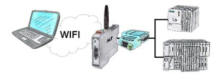
Your're right in the middle of your production line and and should move around the machine and simultaneously observe / manage. No problem, you parameterize the ALF, connect to the S7-LAN and connect to the WIFI-network of the ALF and are ONLINE on the PLC.
