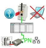
S5-PLC triggered DB-backup/-restore without additional PC via PG-socket and Ethernet on USB-stick
