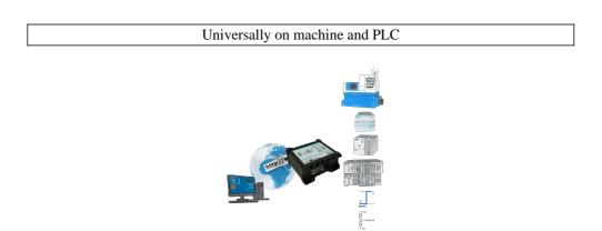
Remote access to all your systems, PLCs without great effort. Even triggering of actions by setting the integrated digital-outputs or reading in the digital and analog-inputs is possible via the Internet connection.
