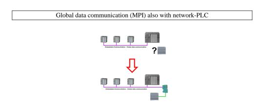
Running global-data-communication between MPI-PLCs (S7-300/400), is one of these PLCs replaced with a newer PLC with network-interface (S7-1200/1500), this PLC was not able to access this data.
