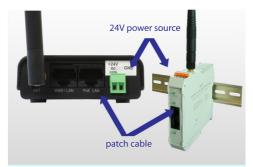
Connect the 24V power source and the computer to configure
