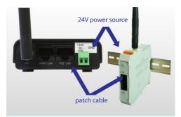
Connect the 24V power source and the computer to configure
