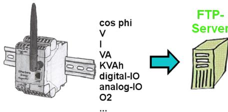
Do you need the logged data not locally but on your site? Then just turn on recording on an FTP-server and the data is stored. You can then immediately read and process this data.
