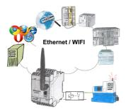
Switch with the EtherSens Control with relay-output easily and directly over LAN or WIFI up to 230VAC/16A, switchable over web-browser, TCP/IP-protocol or PLC-controlled. At the same time you monitor the switching-states on the optional SD-card or on the FTP server.
