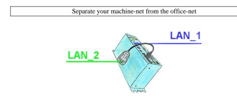
You need a separation between the machine-net and the office-net? No problem, plug a PCMCIA-LAN-card in your Tele-Prof-II-device (only for version -H) and the separation is OK. You have access to both nets via remote maintenance.
