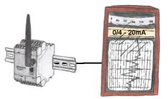
By connecting a line-recorder to the EtherSens-device anyone without network-knowledge can visually capture and further process the log.
