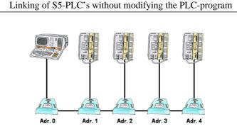
You have to link several S5-PLC's so that in case of need you can respond to all of them without modifying the PLC-program? No problem, connect all PLC's that are in the run with the IBX-Klemme, set up the respective address (1 to 30) at the IBX-Klemme and with the address 0 you will be able to respond to all PLC's via PD-bus-path selection.
