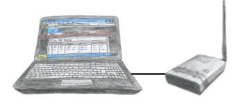
To configure ALF you dont need additional driver or special cables, you connect your PC via LAN or WLAN with ALF and over the integrated webserver you can configure the needed function.
