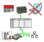
S5-PLC triggered DB-backup/-restore without additional PC via PG-socket and Ethernet on SD-card
