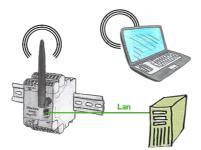
Access parallel via LAN and Wifi to the EtherSens-device. Therefor create via the web-server for each way an ip-address, regardless whether its the same subnet or not.
