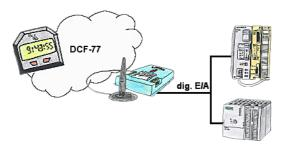
For your production flow you're always in need of an exact time? No problem, connect the SPS-Clock with 4 digital in-/outputs of your PLC, after synchronisation of the SPS-Clock the updating time can be read in a DB of the PLC.
