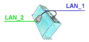
You need a separation between the machine-net and the office-net? No problem, plug a PCMCIA-LAN-card in your Tele-Prof-II-device (only for version -H) and the separation is OK. You have access to both nets via remote maintenance.
