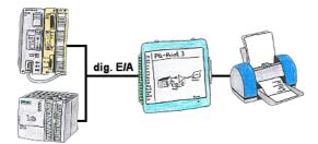
You need production data, circulation lists of your PLC's, but don't want to use a CP or don't get a serial printer anymore? No problem, you need 8 digital outputs and 3 digital inputs of the PLC, and if you connect the PG-Print at it you can generate these lists with a EPSON- or HP-compatible parallel printer.
