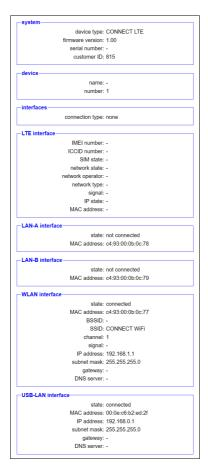
In the Configuration menu, the expert configuration will be carried out differently from the quick commissioning of the device. For example, you can set the DHCP mode, set IP addresses, and carry out the basic configuration of the device again.
