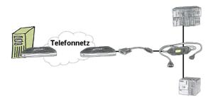
You have to reach urgend your PLC via remote maintenance and have no TS-adaptor in your company? No problem, configure with the MPI-Kabelmanager your S7-interface-cable MPI-II-Kabel the mode "TS" for "remote maintenance", connect this cable with the TS-Adapter (article number 9350-TS) with a standard modem and send it all to your client. Now you will be able to start the connection with your TS-sofware and solve the problem. And this all without buying a original TS-adapter.
