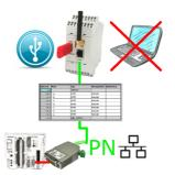
S5-PLC triggered DB-backup/-restore without additional PC via PG-socket and Ethernet on USB-stick
