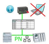
S7-PLC triggered DB-backup/-restore without additional PC via PN-port to USB-stick
