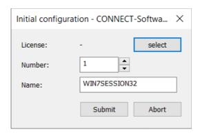
Select the license file that you received by email and accept it, specify the number of the participant, analogous to the numbers of the CONNECT devices. A "device name" can also be specified. This name is then visible in the other devices like a hardware device.
