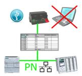
Via digital input triggered DB-backup/-restore without additional PC via PN-port to USB-stick
