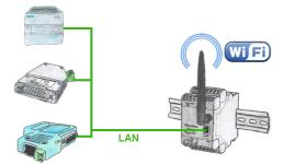
You also need to network devices but dont have locally no ethernet-cable. Wifi is available? With the EtherSens-Bridge you bring immediately all connected wired participants in the WLAN network.
