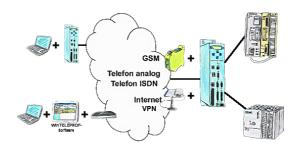
Access to the connected PLC takes place by coupling via Analogue-, ISDN-, mixed Analogue-ISDN-, GSM-, UMTS-line and also via Internet with and without VPN-security.
