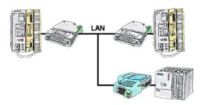
Your pumping stations report the water levels of the central control via telephone network. The central office itself can of course transmit commands/messages to the substations as well. Therefore no dedicated line is required, it's sufficient when the stations connect via network (DSL-router).
