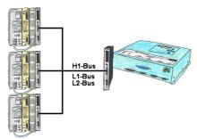
You have an existing L1-, L2- or H1-bus on the customer side and have to program parallel the PLCs? No problem, just connect the communication processor (CP) with a monkey swing to the PLC, the Tele-Network-device with the TELE-CP-cable to a free CP and select the needed PLC with PG-path selection. Herefore the L1-, L2- or H1-option is needed.
