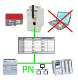
S7-PLC triggered DB-backup/-restore without additional PC via PN-port on SD card
