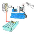
Your installation shows an error and the commissioning engineer isn't available? Connect S5-DIAG with the PLC, enter reason of PLC's malfunction (e.g. O32.5 doesn't come) and the device lists all possibilities why the output has not been set. So you're able to figure out the problem (e.g. safety door not locked) quickly. Finding the cause of the malfunction can be so quick and easy.
