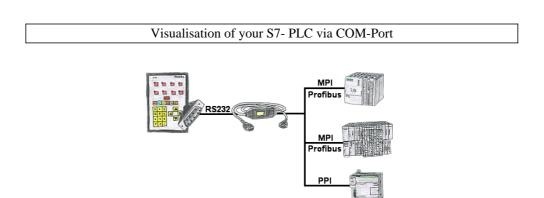
Your panel provides a serial port and no MPI/Profibus for connecting a S7-PLC. Connect the MPI/PPI-cable with it and you're Online with your panel.
