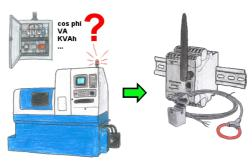
Do you also need the energy-consumption of your plant or need to determine the cos phi? With the EtherSens Energy you can capture and record by using a Rogowski-coil or folding-core the required values.
