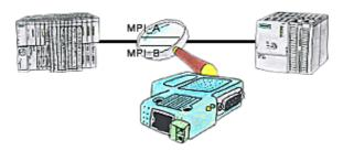
The S7-LAN can also be used for controlling/checking the MPI/Profibus. It will be plugged on the Bus so that you can take a look at the status of the busses via software on PC, for example the numbers of parity errors.
