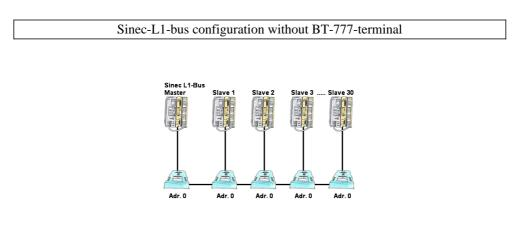
You have to configure a Sinec-L1-bus, own the master, but there's no BT-777-busterminal to buy? No problem, connect the IBX-Klemme to every S5-PLC that is in the run via the optional IBX-SPS-cable, supply every IBX-Klemme with ext. 24V DC if the PLC is not able to provide it, set-up the address 0 and define the actual L1-bus-address in the PLC. Now your master can communicate with the slave-assemblies.
