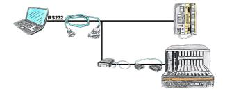
You have a PC with programming software and a 9pin COM-port as interface? No problem, for this purpose the PG-UNI-II-cable is exactly the right product. Connect it to PLC and PC and you're Online. The communication itself is visible by the both included LEDs. Even the 25pin interface of the AS511-card is no problem. You need the NETZ-adapter and also the AG-150-adapter and then this control is programmable, too.
