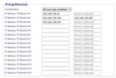
The IP filter is used to determine whether or not the entered IP-addresses or IP-address-ranges may communicate with the connected controllers via the module.
