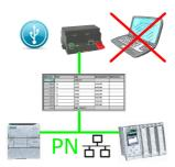
$S7\text{-}PLC\ triggered\ DB\text{-}backup/\text{-}restore\ without\ additional\ PC\ via\ PN\text{-}port\ to\ USB\text{-}stick}$
