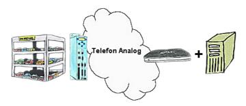
Your car park or control sends the configuration / capacity utilisation to a PC with a modem, so that the data can be used for further processing.
