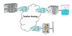
Your pumping stations report the water levels of the central control via telephone network. The central office itself can of course transmit commands/messages to the substations as well. Thereto no dedicated line is required, a "normal" telephone connection is sufficient because the devices hangs up the line after occured message.
