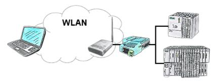
You are on site your plant and should move round the machine and simultaneously control or monitor. No problem, you parametrize ALF as an access-point and connect your S7-LAN or other network-client to him, connect your PC with him and you are online on the PLC.
