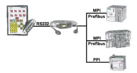
Your panel provides a serial port and no MPI/Profibus for connecting a S7-PLC. Connect the MPI/PPI-cable with it and you're Online with your panel.
