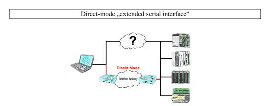
There is an unsupported control or data logger or converter integrated in your installation which protocol is not supported? No problem, the signs that the PC in the office sends will be transferred via telephone line by the Direct-mode , and on-site reproduced by the TP/TB. The way back is identical. So in that case there's also a communication to the electronic devices available.
