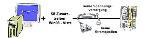
You still have a PC with Win98 and Step5-package and would like to go Online on your S5-PLC via USB? No problem, the provided virtual Com-Port PLCVCom emulates a COM-port on your PC with which you go Online. With a patchtool for the Siemens Step5-software, which is provided as well, nothing else stands in your way to communicate via LAN.
