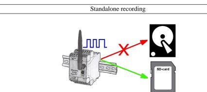
With the integrated SD-card-slot you back-up the recorded data in the device and dont need an external memory. Nevertheless you can send additional the data via FTP to a FTP-server.
