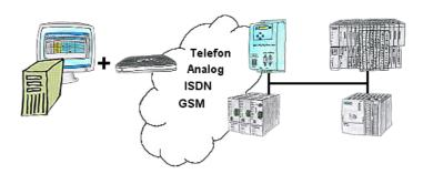
You have to solve a problem in the PLC-program, but the installation is not placed nearby? No problem, start your PG-2000-software with "option teleservice", activate your modem and after selection intra PG-2000-software access to the PLC is possible as if being on-site.
