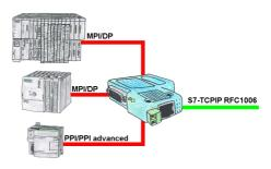
Networking of all S7-controllers (S7-200/300/400), for example with your production-data-acquisition, Industry 4.0 (OPC Server UA or Classic), panels and other devices that communicate via S7-TCPIP RFC1006. One module for all bus-types: PPI, MPI and Profibus.
