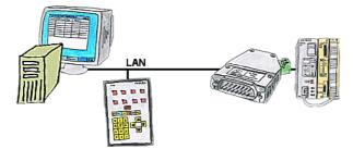
Your panel only has a LAN-socket as PLC-interface, no problem. Connect this socket with the S5-LAN++ and plug it directly on the PD-interface of the PLC. Then access to the variables and data of the PLC is already available.
