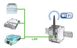
You also need to network devices but dont have locally no ethernet-cable. Wifi is available? With the EtherSens-Bridge you bring immediately all connected wired participants in the WLAN network.
