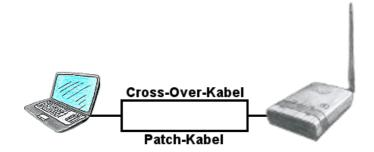
You need ALF to connect to a reachable WLAN, but only have a patch-cable? No problem, ALF provides "autonegotiation" and this means that he recognises a connected cable (patch-cable or cross-over-cable) and surround the pinning according to the cable, so a communication is possible.
