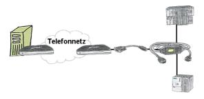
You have to reach urgend your PLC via remote maintenance and have no TS-adaptor in your company? No problem, configure with the MPI-Kabelmanager your S7-interface-cable MPI/PPI-Kabel the mode "TS" for "remote maintenance", connect this cable with the TS-Adapter (article number 9350-TS) with a standard modem and send it all to your client. Now you will be able to start the connection with your TS-sofware and solve the problem. And this all without buying a original TS-adapter.
