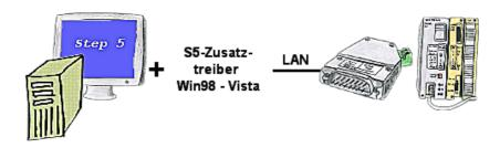
You still have a PC with Win98 and a MS-DOS-based Step5-package and would like to go Online on your S5-PLC via LAN? No problem, the provided virtual Com-Port PLCVCom emulates a COM-port on your PC with which you go Online. Even your MS-DOS-based Step5-software on this WIN98-PC can use this virtual Com-Port. With a patchtool for the Siemens Step5-software, which is provided as well, nothing else stands in your way to communicate via LAN.
