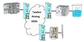
Your pumping stations report the water levels of the central control via telephone network. The central office itself can of course transmit commands/messages to the substations as well. Thereto no dedicated line is required, a "normal" telephone connection is sufficient because the devices cut the line after occured message.
