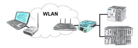
You are on site your plant and should move round the machine and simultaneously control or monitor. WLAN is reachable, but your PC is not able to provide WLAN. No problem, you parametrize ALF as a client and connect him to the PC and join the reachable WLAN and you are online on the PLC.
