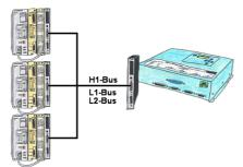
You have an existing L1-, L2- or H1-bus on the customer side and have to program parallel the PLCs? No problem, just connect the communication processor (CP) with a monkey swing to the PLC, the Tele-Network-device with the TELE-CP-cable to a free CP and select the needed PLC with PG-path selection. Herefore the L1-, L2- or H1-option is needed.
